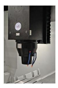
IMPROVEMENT – Spindles are equipped with a Fast-acting tool drawbar gripper. This device has a pre-hold system that allows the tool clamping to be finalize during spindle disengagement from tool change position.
