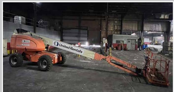
JLG 660SJ Boom Lift
