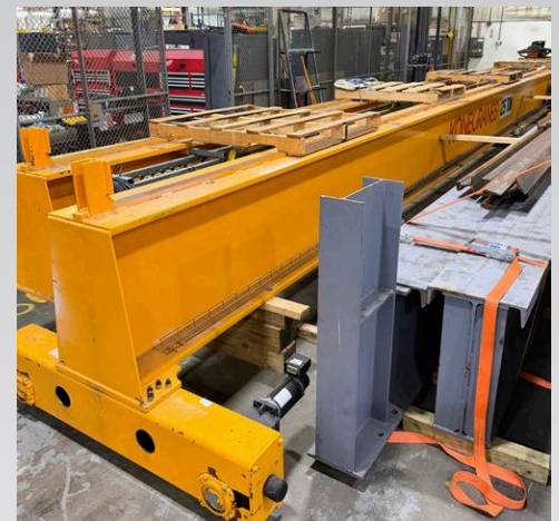
25-Ton Konecranes Freestanding Bridge Crane System (Disassembled)
