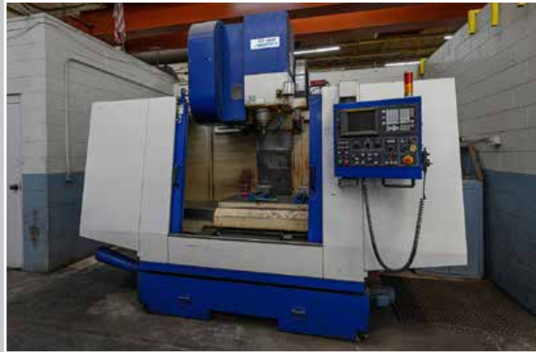
JOHNFORD SV-45H CNC Vertical Machining Center
