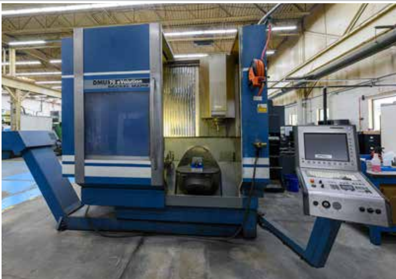
DMG Deckel Maho DMU 70 eVolution 5-Axis CNC Vertical Machining Center
