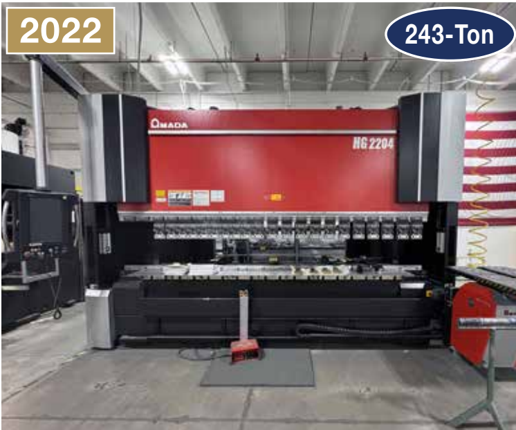
AMADA HG2204-M15H CNC Hydraulic Press Brake
