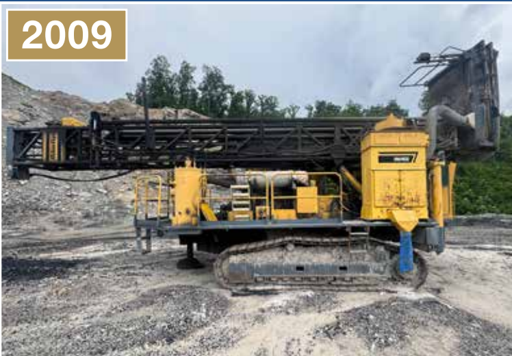
ATLAS COPCO DM45E Drilling Rig
