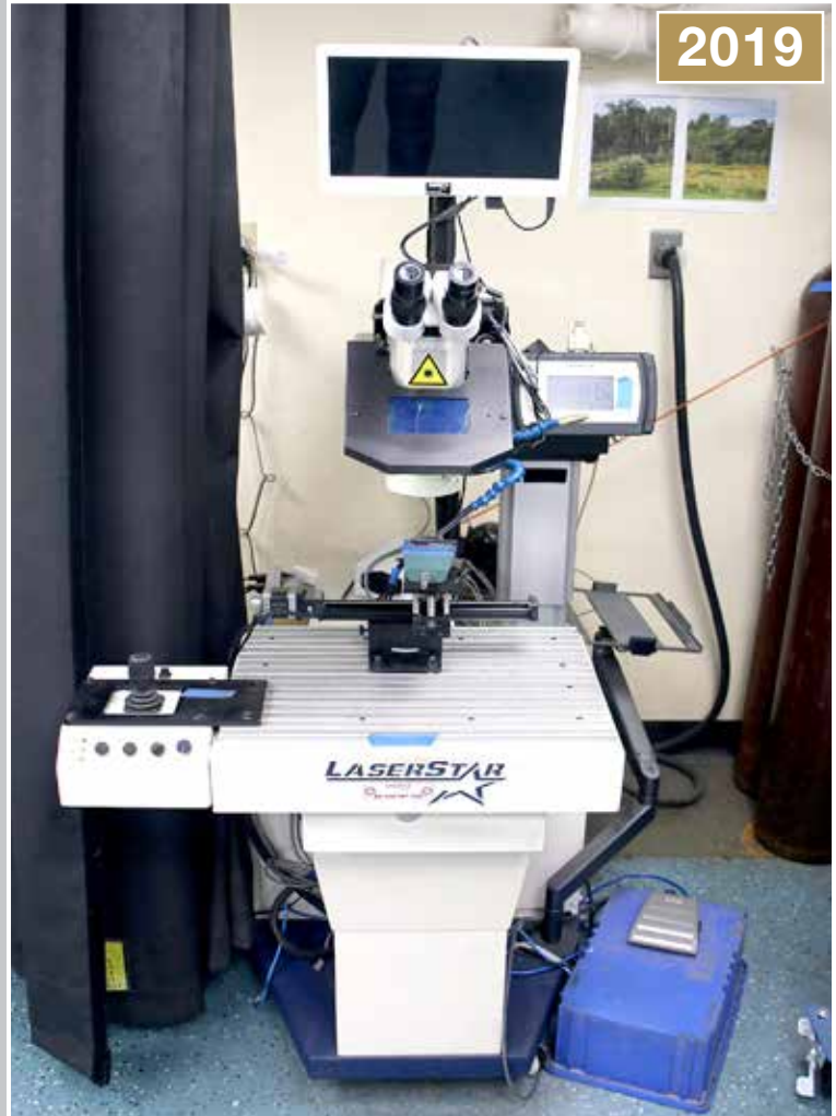
LASERSTAR 513-786-150-1-MD Fiber Optic Laser Welder
