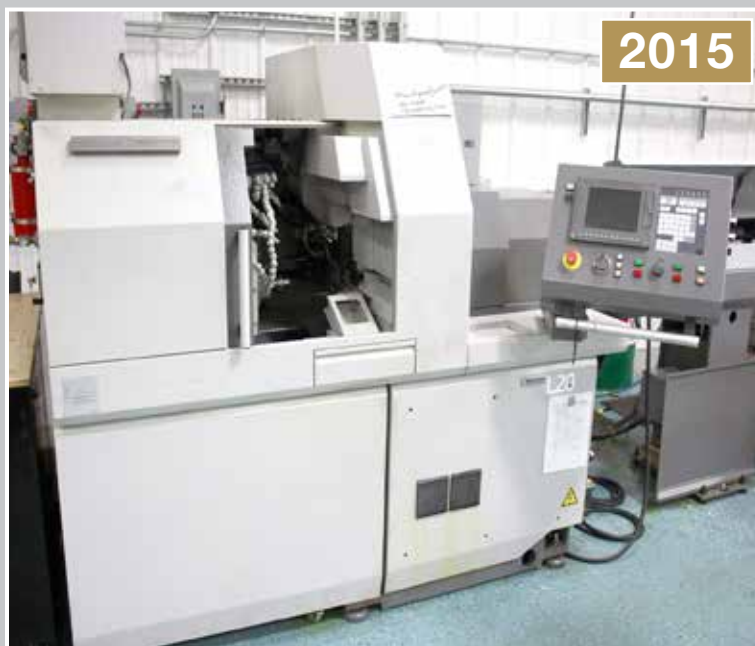
CITIZEN L20E-2M8, 7-Axis CNC Swiss Type Auto. Screw Machine
