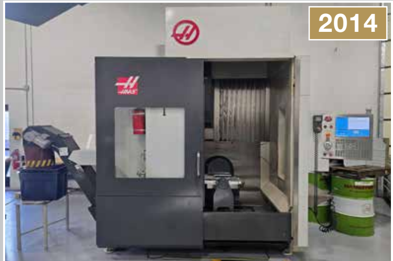
HAAS UMC-750 5-Axis CNC Vertical Machining Center
