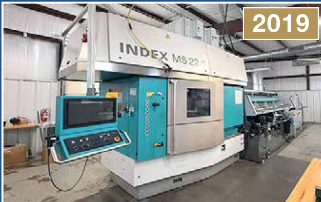
INDEX Multi-Spindle Horiz. CNC Screw Machine
