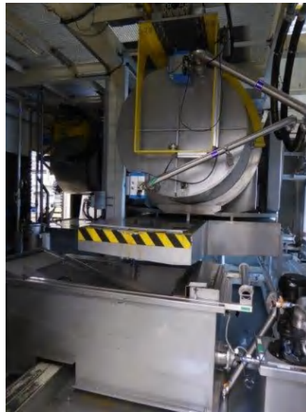
e) OP 30 MTM OMEGA 4-H, 4-chamber rotary transfer washing unit
