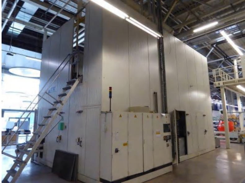
e) OP 30 MTM OMEGA 4-H, 4-chamber rotary transfer washing unit
