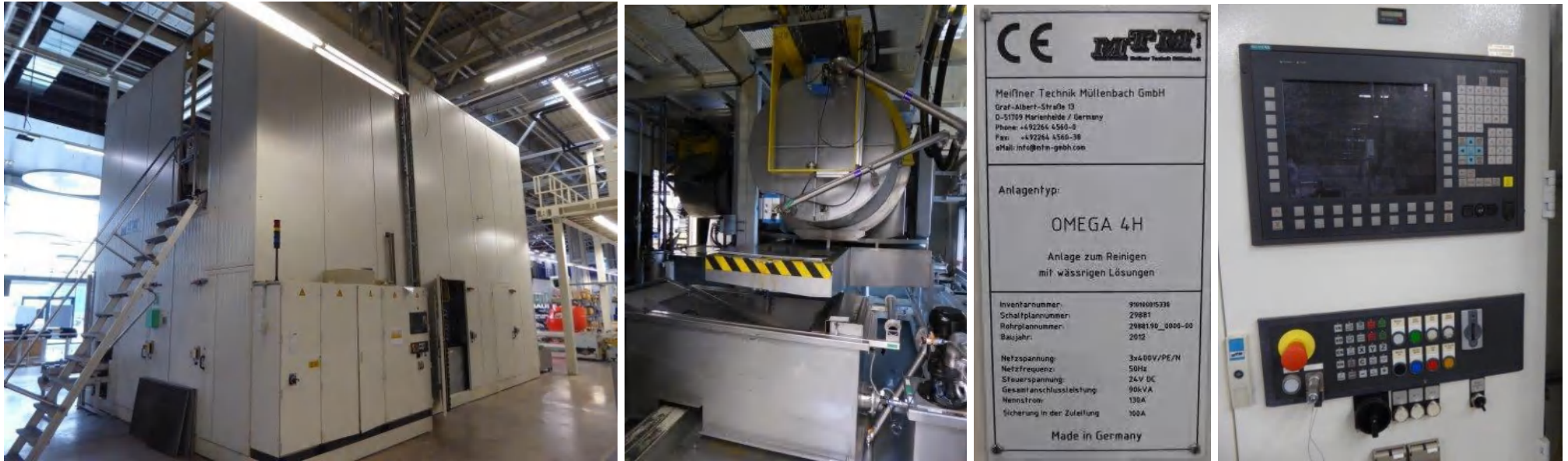
e) OP 30 MTM OMEGA 4-H, 4-chamber rotary transfer washing unit
