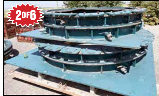
TBM Launch Seals
