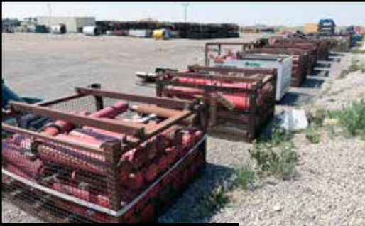
Intermediate Jacking Cylinders
